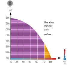
Maximum working pressure 40 bar at 70°C
