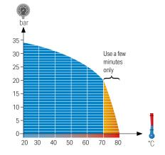
Maximum working pressure 20 bar at 70°C
